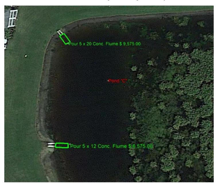
Agenda Page #55 Lake "C" Install up to 20 Ft. of Re-grading Slope, Install of High Flow Fabric with 3 to 6 Inch Rip Rap
