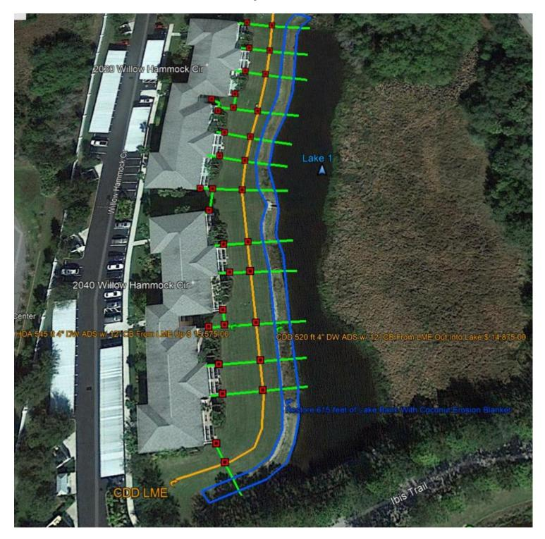
Agenda Page #52 Lake 3: 30 Feet of Lake Bank Erosion Repair with Coconut Erosion Blanket.
